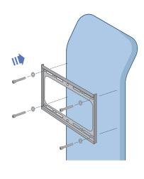
Screw the TV Mount on the display using the M6 Screws and M6 washers.
