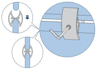
Tighten the clamps with the allen key to secure the header in place.
