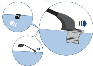
To avoid stripping the light clips, do not twist the knobs too tight.
