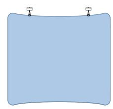
You can adjust the frame alignment by having a person on each side gently shift the top corners until the display stands completely straight.
