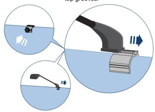
To avoid stripping the light clips, do not twist the knobs too tight.
