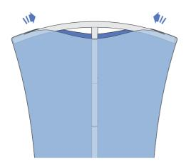
For the straight model, shorten the profile before lifting the fabric.
