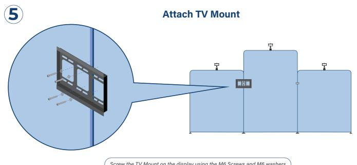
Screw the TV Mount on the display using the M6 Screws and M6 washers.
