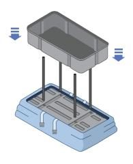
Install the Poles into the Case Lid, then install the Storage Case.
