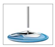
4. Fit the uni-pole to the base by sliding it on.
