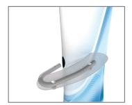
9. Slide shelve through the open slit in the print and fit it on the support socket.
